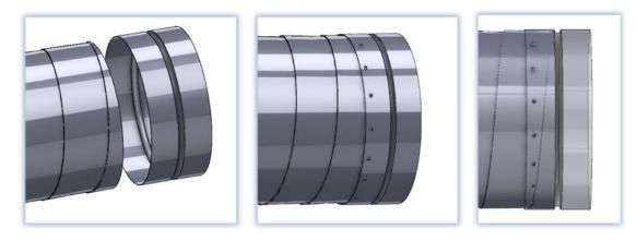
• Flanged connections (for ducts OTF), by applying a layer of sealing material (e.g., PVC stripe) to the brim of the flanges and tightening them with bolts.
