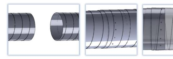
Connection of ducts with external couplings (LMF). When using this type of connection, special sealant is needed, because there is no rubber gasket. Fastening with self-tapping screws or rivets.
