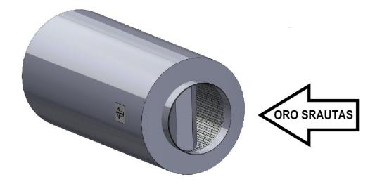
In case the silencer is being installed close to the inlet/outlet, ensure no precipitation gets inside. If the noise dampening material gets wet, the silencer will no longer perform its function.
