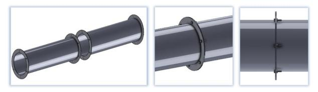
The fastening elements, used for connection of parts, (screws, rivets) should be spread out evenly around the perimeter. To achieve better tightness, it is recommended to use special sealant or silicone for ventilation.
