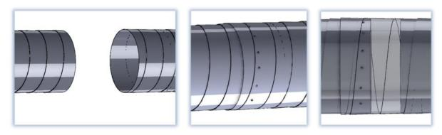
Connection of ducts with external couplings (LMF). When using this type of connection, special sealant is needed, because there is no rubber gasket. Fastening with self-tapping screws or rivets.
