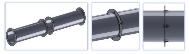
The fastening elements, used for connection of parts, (screws, rivets) should be spread out evenly around the perimeter. To achieve better tightness, it is recommended to use special sealant or silicone for
