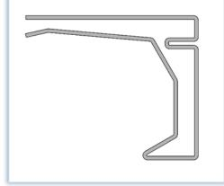
When connecting the ducts, a sealing gasket is glued between the flanges. The gasket should be uniform around the whole perimeter of the flange and also not cover the fixation holes. Corners of the flanges are joined together with bolts and the flanges are clamped together by C type profile or by joint clamps.
