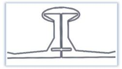
C type profile is slid over the whole length of the flange profile. Joint clamps are fastened at each 250 mm length section of a flanged connection (minimum 1 joint clamp per one side).
